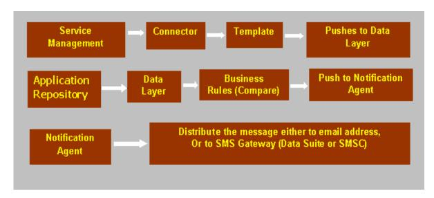
Administrators will start the **HexaALERT** through the Service Manager. The Connector component will connect to the SAP Logical and Oracle Database Layer, which abstracts any database available, and polls for data (events) from the Database Layer as per details set in the Templates. The data received from the Database Layer will be pushed to the Data Layer, which holds the data in a device independent format.
